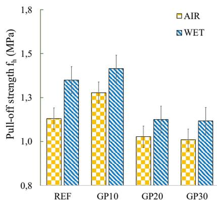
Fig.4 Average pull-off strength  $f_h$  of the subsurface layer.
