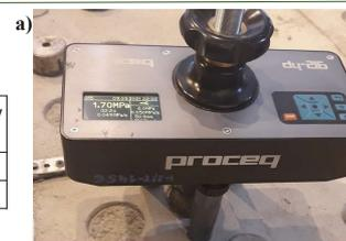
Fig.2 Pull-off strength  $f_h$ , a) test device, b) test in cross-section
